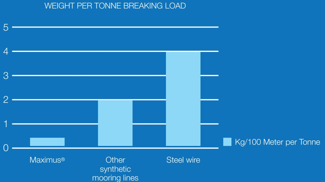
Testimonials from crews on our customers' vessels confirm the ease of use of Maximus®. Maximus® not only allows for efficient and timely mooring thanks to its weight, the unique composition of the rope also allows for a safer mooring solution.
